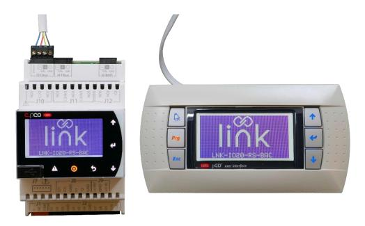
The external display can be used as a commissioning tool, to facilitate the operation of an engineer on site, having a hand-held display available to use.
