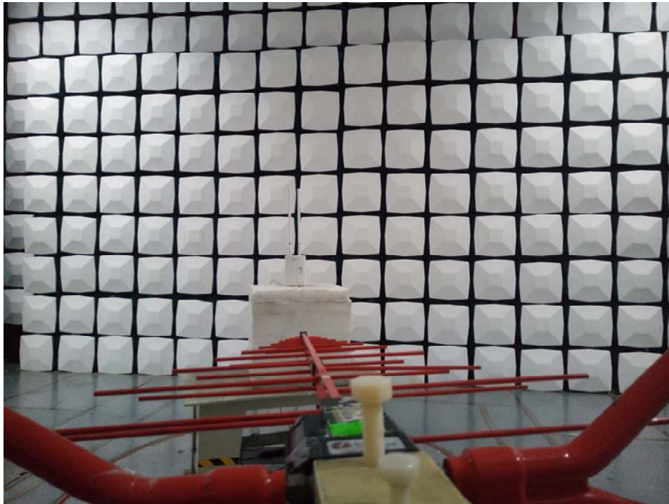
Radiated Spurious Emissions Test View Above 1GHz
