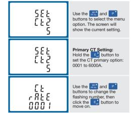
Hold the E button to save your adjustment. Hold the way button for 3 seconds to exit the set up menu.
