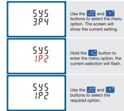
Hold the E button to confirm your adjustment. Hold the with button for 3 seconds to exit the set up menu.
