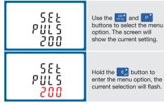
Use the  $\mathbb{P}_{\text{Fite}}^{\text{MDA}}$  and  $\mathbb{P}_{\text{I}}^{\text{MDA}}$  buttons to choose the desired pulse rate. To save the new setting, hold the  $\mathbb{E}_{\cdot}^{\text{MDA}}$  button for 3 seconds until the selection stops flashing.
