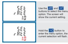
Use the with and buttons to choose the desired pulse rate. To save the new setting, hold the c button for 3 seconds until the selection stops flashing
