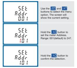
Use the way and puttons to choose the necessary number, then press the c button to move along to the next number. To save the new setting, hold the c button for 3 seconds until the selection stops flashing
