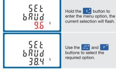
On completion of the entry procedure, hold the E button to confirm the setting.
