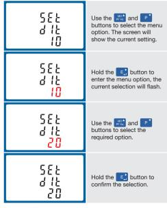
Hold the *w* button for 3 seconds to exit the set up menu.
