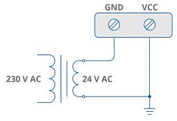
Figure 5. AC power connection
