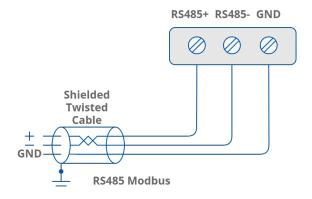
Figure 6. Communication bus connection
