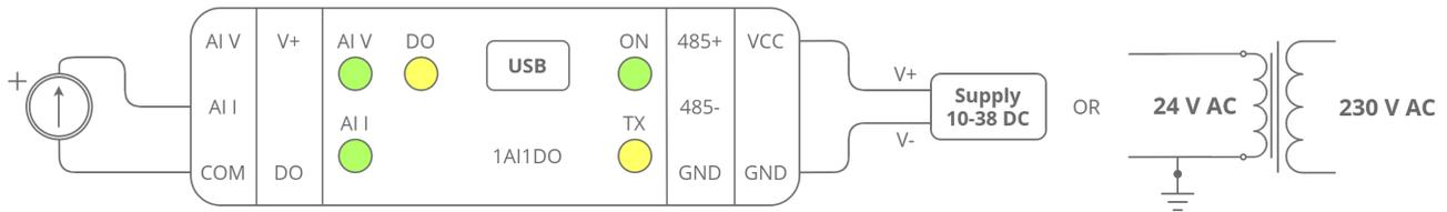
Figure 8. Connection of current measurement
