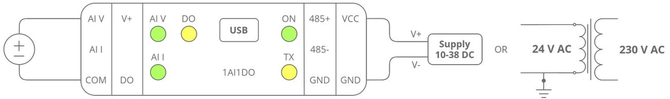
Figure 7. Connection of voltage measurement
