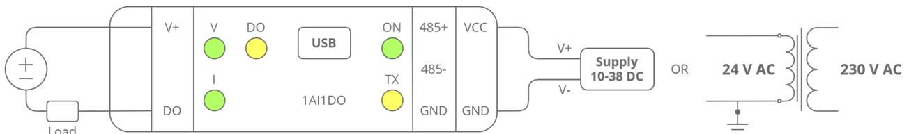
Figure 9. Connection of PNP type digital output
