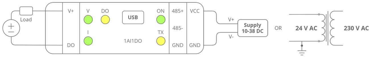
Figure 10. Connection of NPN type digital output
