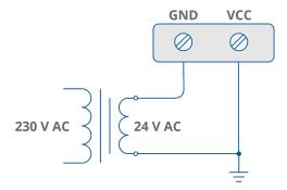
Figure 5. AC power connection
