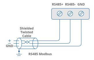
Figure 6. Communication bus connection
