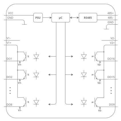
Figure 3. Block diagram
