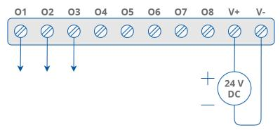
Figure 8. Connection of output
