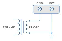
Figure 5. AC power connection
