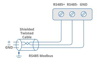
Figure 6. Communication bus connection
