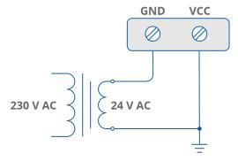
Figure 5. AC power connection
