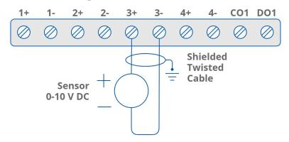
Figure 8. Connection of voltage measurement
