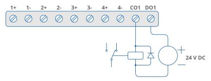
Figure 9. Connection of PNP output
