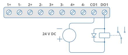
Figure 10. Connection of NPN output
