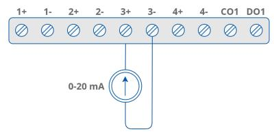
Figure 7. Connection of current measurement
