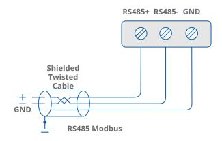
Figure 6. Communication bus connection
