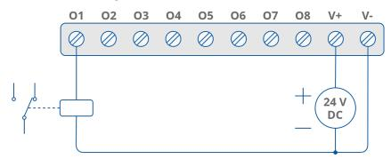
Figure 10. Connection of relay
