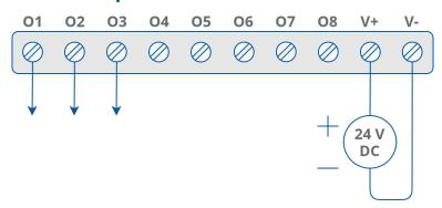
Figure 9. Connection of digital outputs
