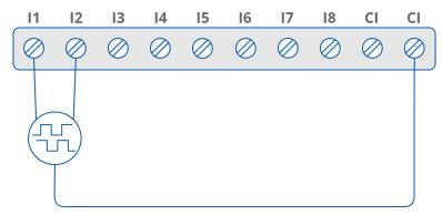
Figure 8. Connection of encoder
