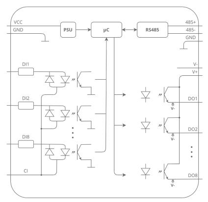
Figure 3. Block diagram
