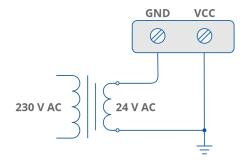
Figure 5. AC power connection
