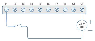
Figure 7. Connection of input
