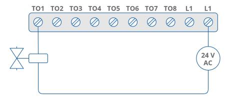
Figure 7. Connection of electrovalve
