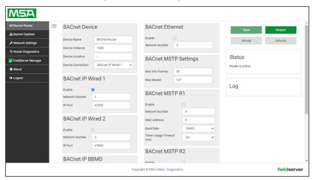
NOTE: For BACnet/IP, click on the Settings button on the left side of the landing page to ensure the BACnet Router is on the BACnet/IP network subnet to configure BBMD.
