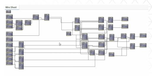
The Deterministic Runtime Engine\* enables deterministic timing when servicing the IO, as well as fast startup times. Create deterministic applications in wiresheet as you would in normal Niagara applications.
