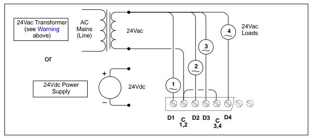
Note that 15-position DO connector plug has 5 common terminals "C" (1–2, 3–4, 5–6, 7–8, 9–10), which are isolated from each other. This can be useful when powering loads from different 24Vac sources.
