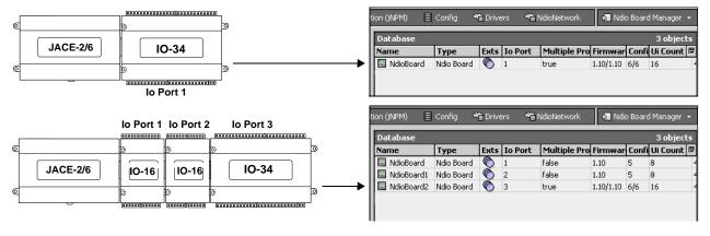
Once the operating system identifies the NDIO processors, the I/O board Status LED on each IO module turns green. The green board Status LED means that the JACE is able to communicate with the I/O. It does not indicate anything about the status of the Niagara station or its Ndio components. See Figure 2 on page 6 for location of the IO-34 board Status LED.
