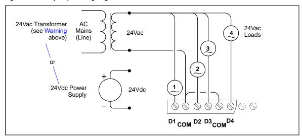
Figure 8 Relay output wiring diagram.
