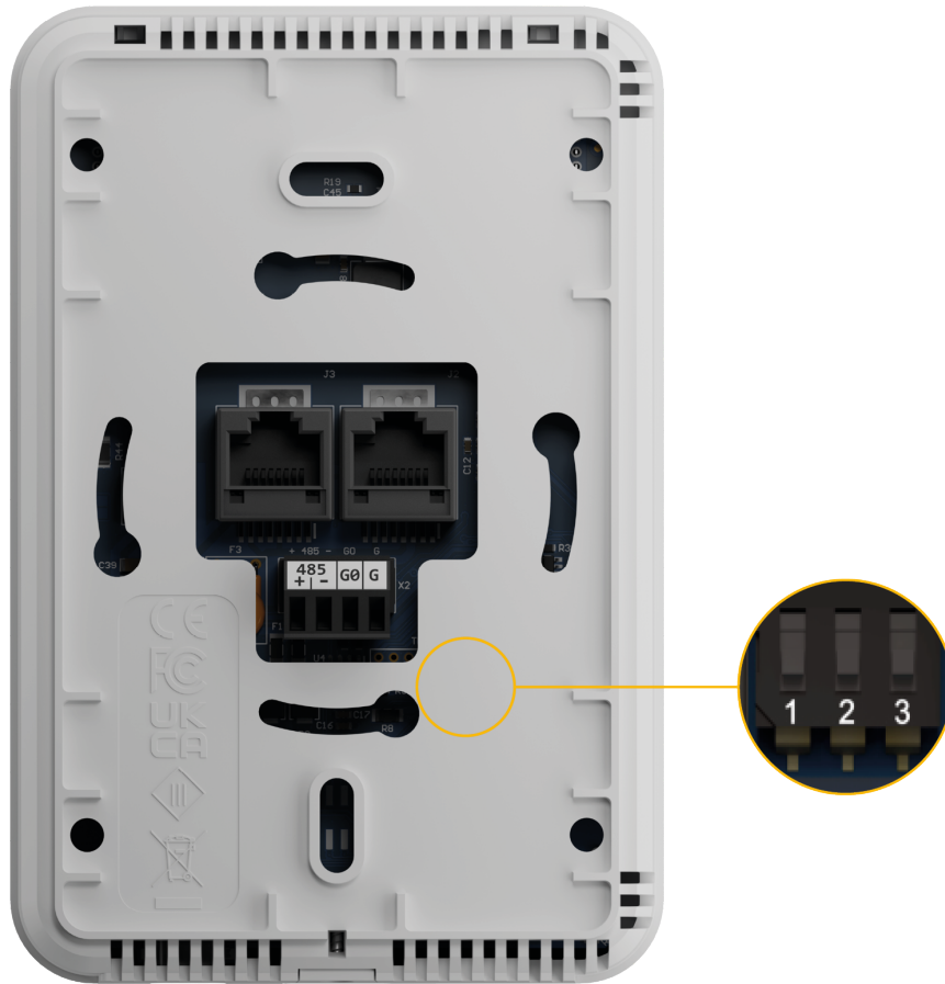
Figure 12. The DIP switch location under the back cover
