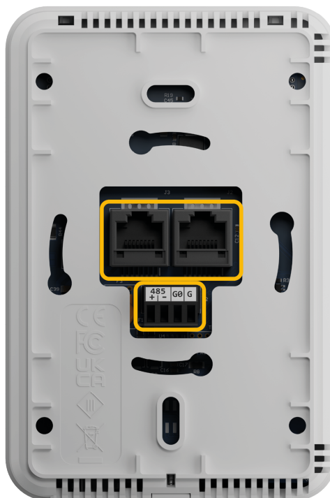
Figure 9. RJ45 connectors and RS485 screw terminal
