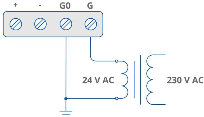
Figure 13. AC power supply connection
