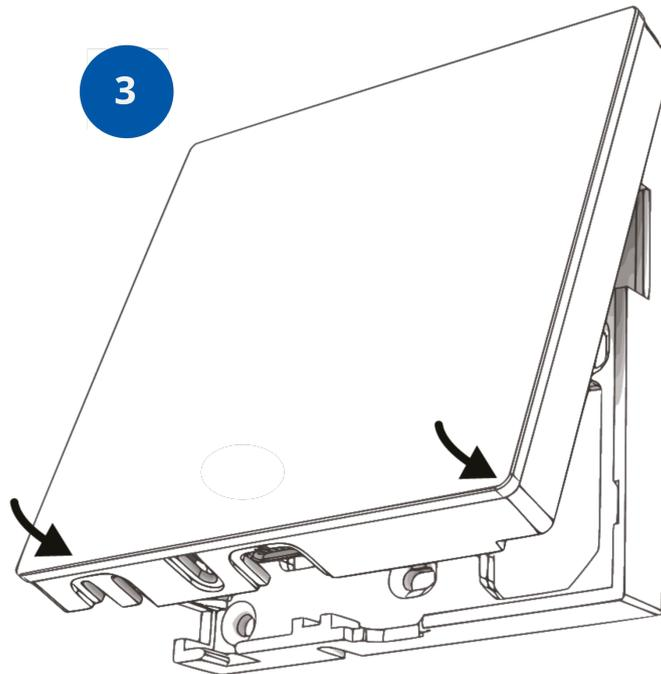
Figure 24. Fitting down corners in the back box
