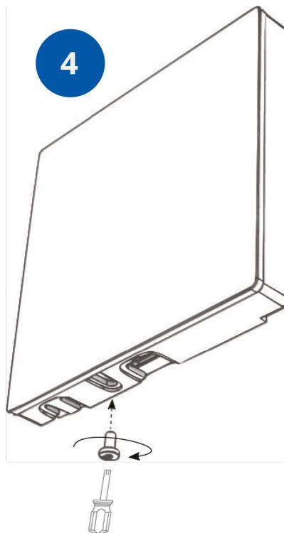
Figure 25. Screw the panel to the back box
