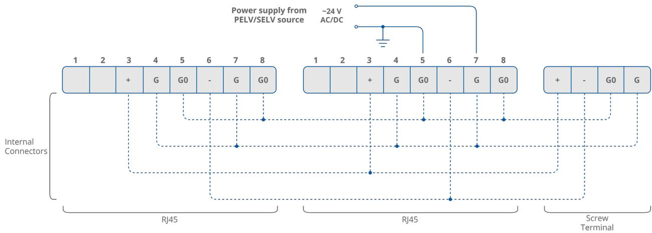
Figure 14. RJ45 power supply connection
