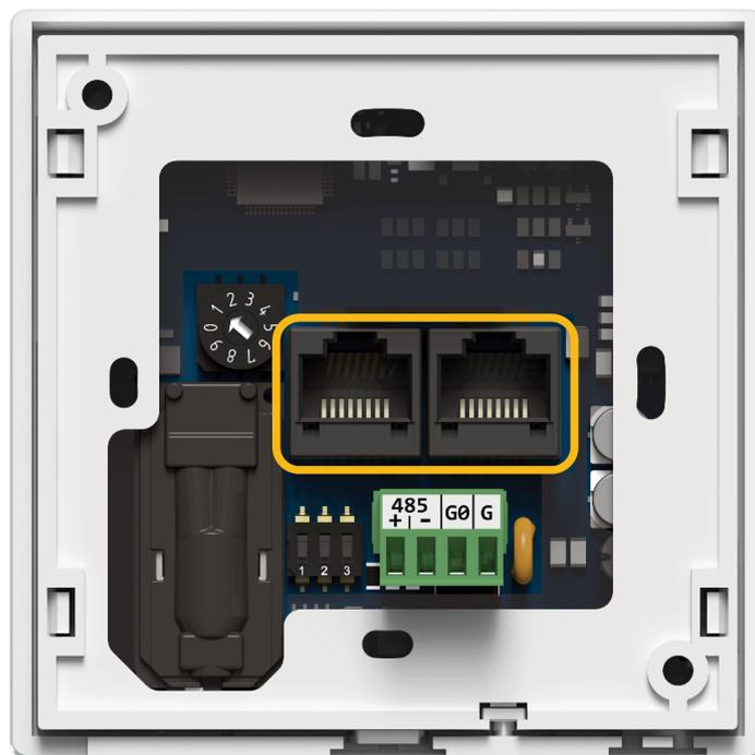
Figure 15. RJ45 connectors
