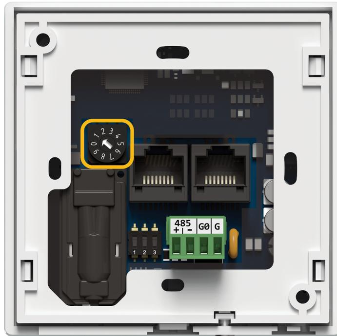
Figure 21. Rotary switch location
