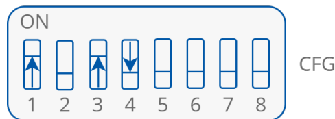
Figure 37. The CFG DIP switch configuration for digital control mode
