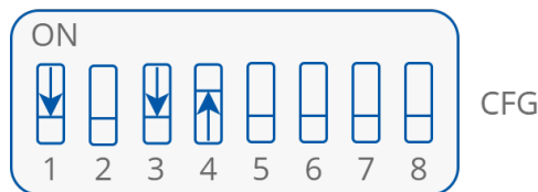
Figure 33. The CFG DIP switch configuration for analog control mode
