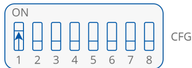
Figure 17. 2-pipe DIP switch configuration
