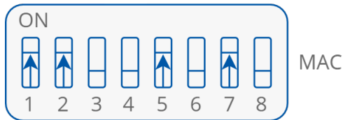
Figure 14. MAC DIP switch settings
