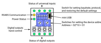
mini USB Switches for setting the device address Address = S2\*10 + S1
