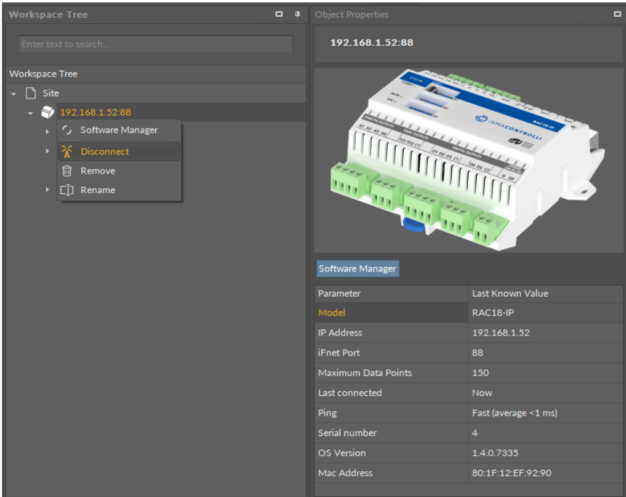
Figure 114. Disconnect option in the context menu of a nano EDGE ENGINE device
