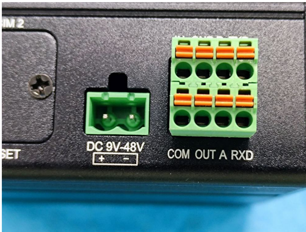
EUT- Port view for model UR35-L04EU-G-P-W
