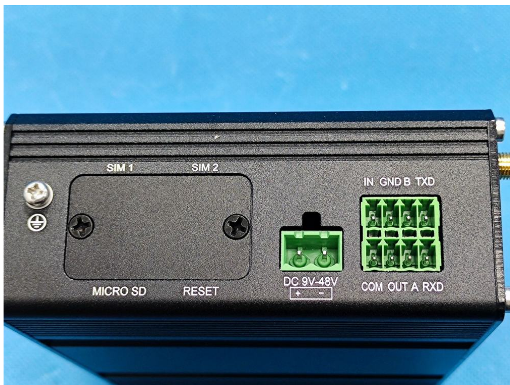
EUT- Port view for model UR35-L04EU-G-P-W-485
