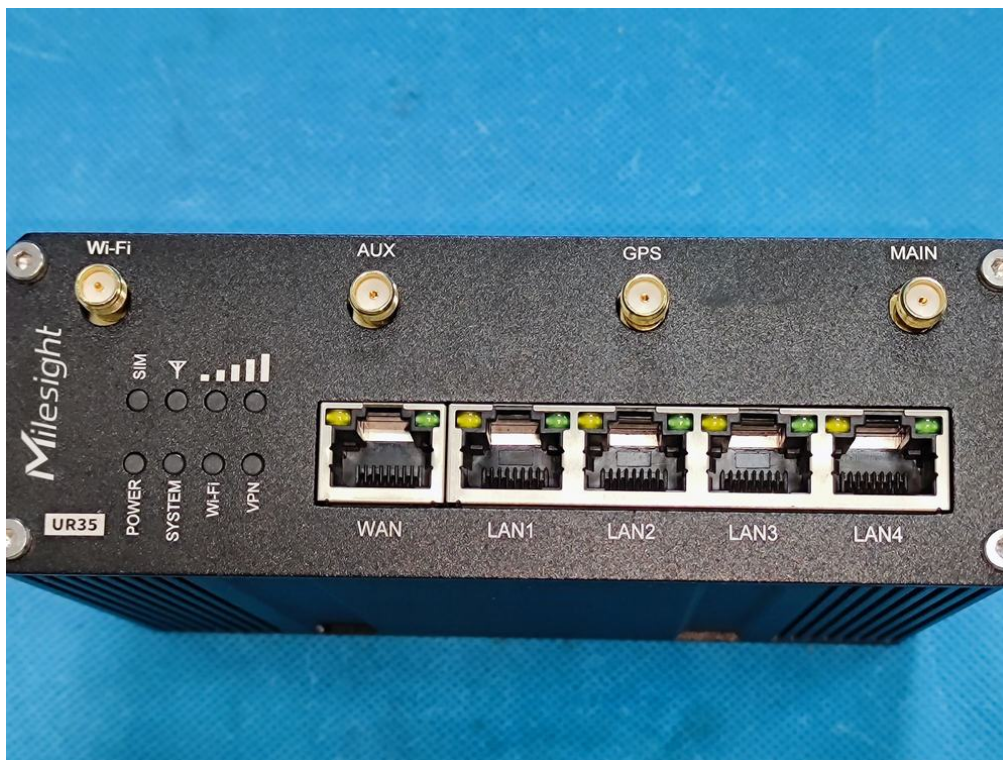
EUT- Port view for model UR35-L04EU-G-P-W
